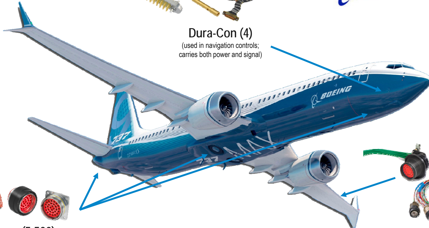
Omega (5,500) (general avionics connector for power and signal; used throughout aircraft – undercarriage deployment hydraulics, flight controls, navigation, mechanical systems and lighting)
